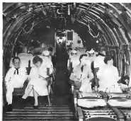
LOOKING FORWARD in the CAB, you see the passengers looking backward. When not in use, the seats are folded flat, as shown, into an open-air walk.
